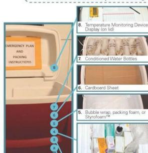
**Close lid** – Close the lid and attach DDL display and temperature log to the top of the lid.
